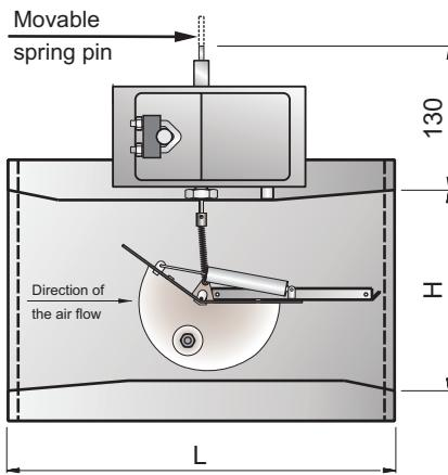
Ref. no. 504: Similiar to ref. no. 503, additional auxiliary switch for activation of an additional switching command.
